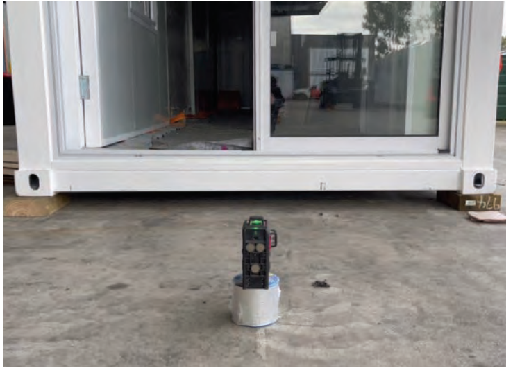
Plane laser on short edge
