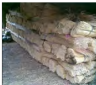
Figure 6. Thatching materials shall be stored such that: 1. the stem surface is not physically damaged, 2. the bundles are clear off the ground, 3. the bundles are not unduly exposed to moisture and the sun.
