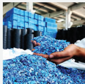
Figure 9: Plastic waste (resin pellets) in reference to the research being conducted by the University of Bath in India by incorporating plastic aggregates in concrete. Source: "Cement's solution to plastic waste," (2018)
