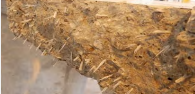
Reinforcing concrete with recycled plastic
