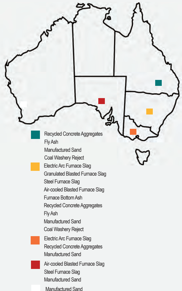
Figure 2: Representing the locations for various recycled aggregates, manufactured aggregates and waste by-products within Australia. Designed by Richter, E. Original/ Information source: Use of Recycled Aggregates in Construction. Cement Concrete & Aggregates Australia (2008).
