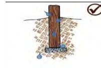
Figure 7. STAND: If a pole is planted on top of a concrete base make sure the base is completely dry before the pole is planted.
