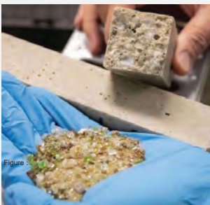
Figure 6: Australian researchers from the University of Melbourne produced eco-friendly concrete from glass waste. Source: Ngo, Tuan; Kashani, Ali; Hajimohammadi, Ailar; and Crough, Damien, "Case study – Using recycled glass fines in light weight concrete," Published by Sustainability Victoria, (April, 2018)
