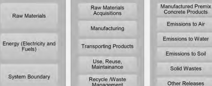
Figure 5. Premix Concrete's Process and Impacts on Environment.
