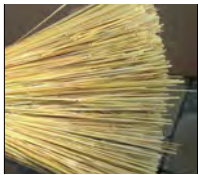
Figure 4. Properly harvested thatch free of any loose material.
