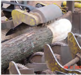
1. Bucking & Debarking Mechanical removal of bark from the logs to then cut them to proper length so as to create peeler blocks. Co-products include bark and wood waste.
