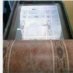
3. Sheet is cooled - dry the ink - coat the top layer - create texture
