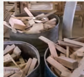
2. Division & Classification Waste timber is classified into Class A (untreated high quality timber) and Class B (untreated and unstained engineered wood products) prior to processing.
