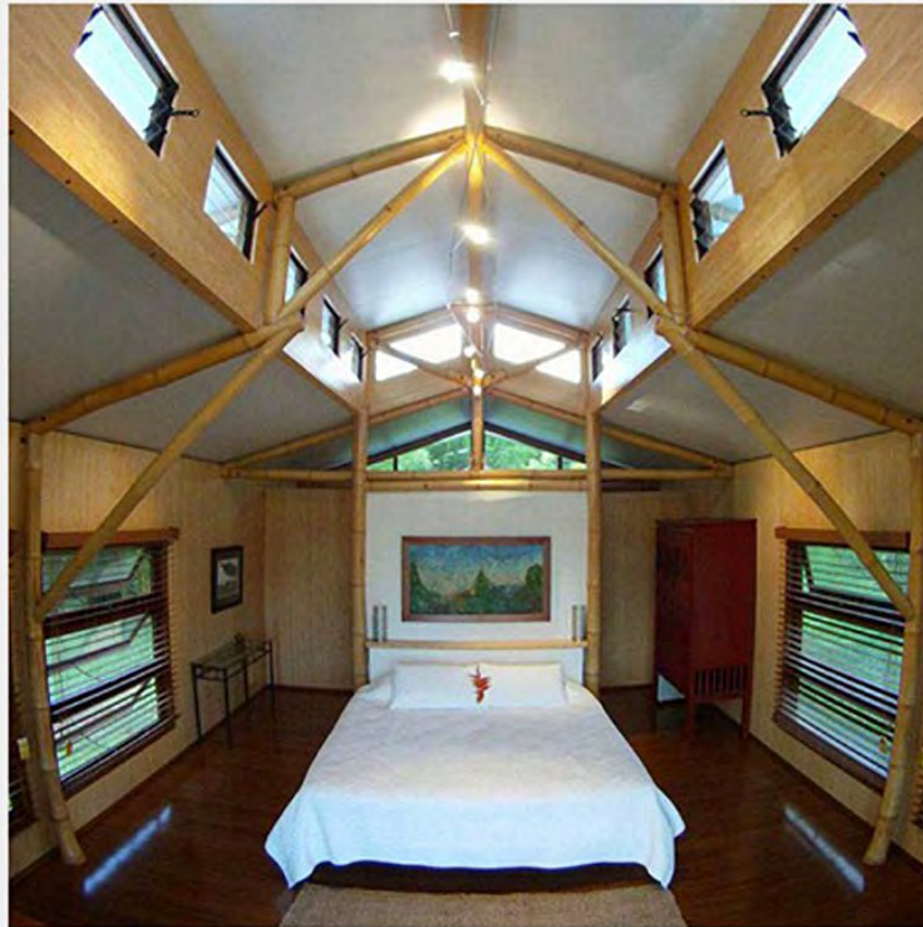
The prototype 'Boo Cottage' (left and top) in Bangalow NSW, created by Barefoot Design, involved the harvesting of over 200 bamboo poles for the modular structural panels, flooring and furniture panels. Images: Jaye Irving, Barefoot Design.
