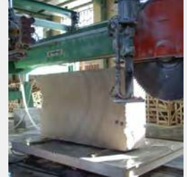
4.Preliminary shaping Cutting stones into blocks
