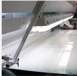
2. Sheet is formed - solidifies the liquid foam - felt paper backing - floors design will be printed directly on this foam
