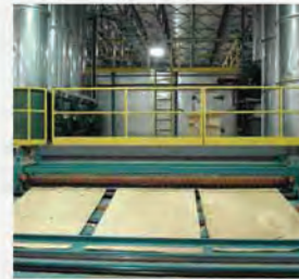
3. Veneer Processing Log are peeled through a veneer lathe to create uniformly thin sheets. Dryers remove the moisture content from green veneer through energy intensive process.
