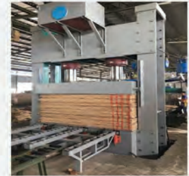
4. Hot Pressing & Sawing Veneers are coated with phenol-formaldehyde resin, subjected to cool pressing for flattening and stacked into panels for hot-pressing. Panels are trimmed and sanded for use.
