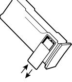
Ensure that the lithium 9V battery has not expired.
