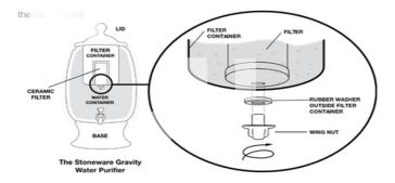
Water is placed in the top container, shaped like an inverted bell, which houses the ceramic filter which has a nozzle protruding through a small hole into the main body of the purifier (please refer to illustration). Once the water passes through the filter it accumulates in the water container where it can be accessed by pressing down on the tap. Water is filtered naturally in three ways.
