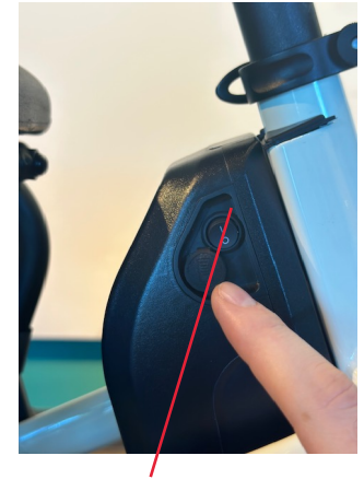
Battery On switch
