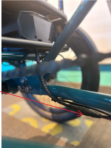
Quick Disconnect (next to the battery)
