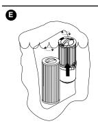
Lift unthreaded filter cartridge from skimmer well.
