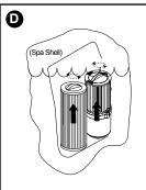
Rotate each filter cartridge handle counterclockwise to unthread from mating wall fitting.
