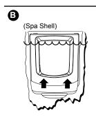
Lift upward on filter cover to release it from the mating retaining clips. Then tilt forward to remove and access filter cartridges.
