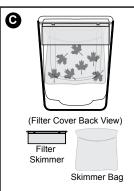
Remove skimmer bag and filter skimmer from clips, then clean out debris. Replace the filter skimmer about every three months, depending on spa use.
