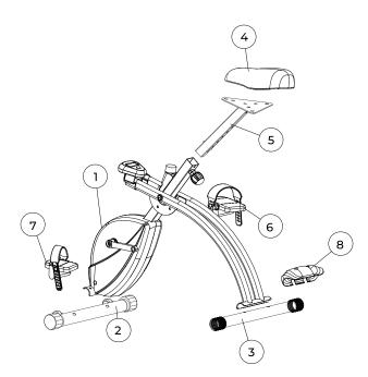
Place the bike frame (#1) in an upright position, insert the included pin (G) into the hole below the pivot point.
