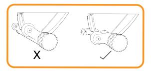
NOTE: When attaching Front Foot (#3) to the Bike Frame (#1) ensure wheels are parallel to the floor, as picture above.
