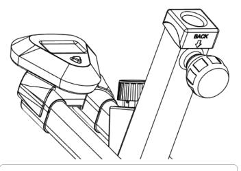
Apply pressure to the sleeve until its fully inserted into the bike frame.
