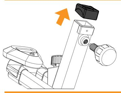
Remove black pastic cap and back off adjustment knob all the way by screwing out counter-clockwise
