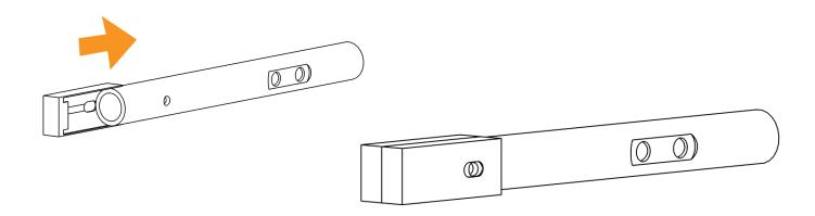
Insert aluminum tube (2) into the seat post (NOT BIKE FRAME)
