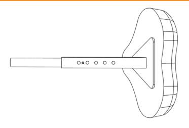
Line up the hole on the aluminum tube with the hole on the seatpost
