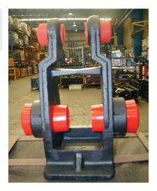
Insert both equaliser bushes in the equaliser hanger bracket tapered bore.
