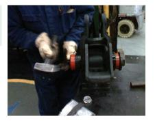
Locate the equaliser in the equaliser hanger. With a nylon faced hammer, tap both of the torque arm and equaliser bushes into position.
