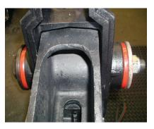
The equaliser assembly is now completed. Note that the equaliser is installed centrally in the hanger bracket and the equaliser hanger respectively. The bush protrusion on the outer ends is consistent see photo for reference.
