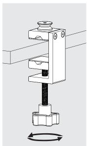
Use the Handle to clamp the component onto the surface.
