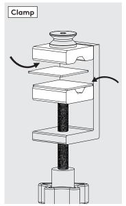
Stick the Rubber **B**1 Adhesive Pads onto the Clamp faces.
