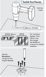
Drill 4x holes with a 4mm drill bit or a 6mm bit. Then fasten the Baseplate as detailed using a Screwdriver.
