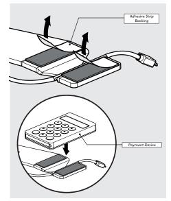
Remove the backing from Adhesive
