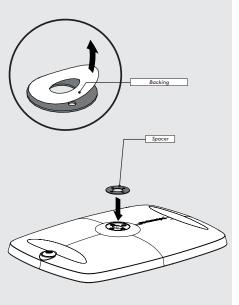
Remove the backing from the Spacer. Align with the screw holes on the Case and firmly stick down.
