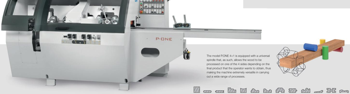
The model P.ONE 4+1 is equipped with a universal spindle that, as such, allows the wood to be processed on one of the 4 sides depending on the final product that the operator wants to obtain, thus making the machine extremely versatile in carrying out a wide range of processes.
