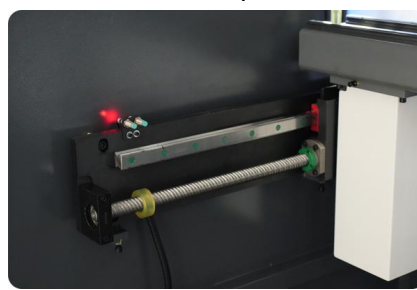
Backgauge use ball screw and linear guide rail
