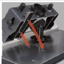
Precision Spindle moulder fence "230", Multi-adjustment system
