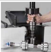
Moulder spindle Quick change system
