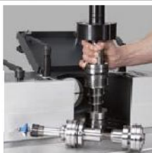
Moulder spindle Quick change system
