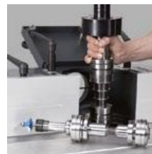
Moulder spindle Quick change system
