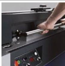
Synchronous opening of the planing tables
