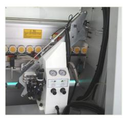
Fast move back structure, move backward while doing full bevel edge, move forward while doing half bevel edge so as to achieve fast switch between bevel edge and straight edge banding work but without possible collision or damage on edge tape.
