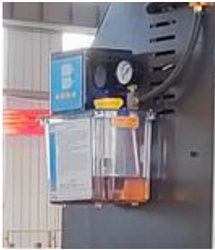
Lubricating system: Automatically oil the guide rails, protect the guide rails in some degree
