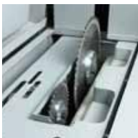
Saw carriage with main and scoring unit
