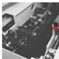
Saw carriage with main and scoring unit
