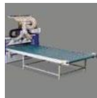
Automatic unloading unit including electric motor driven offloading pusher
