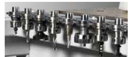
1 tool changer 8- or 11 position tool changer on the side of the machine chassis
