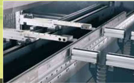
Backgauge with X-, R- and Z1+Z2-axes
