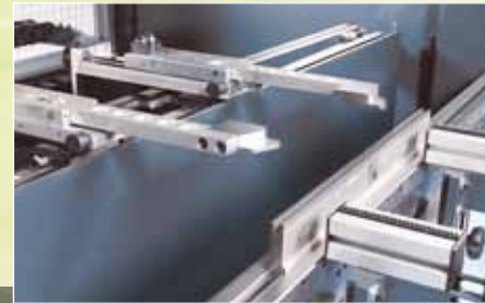
Backgauge with X-, R-, Z1+Z2- and Delta X-axes
