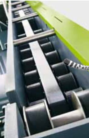
Roller drive with 2 servomotors
