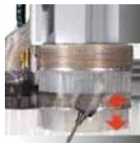
Variable position controlled extraction hood
