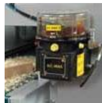
Automatic central lubrication system
