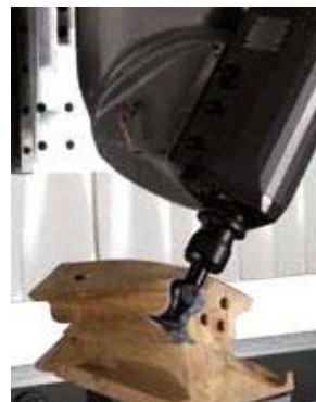
Simultaneous 5 axes processing 3D applications
