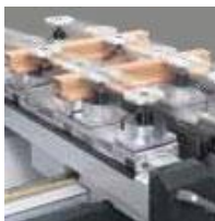
Automatic consoles and vacuum positioning
