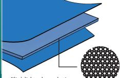
Elite's lighter, longer lasting more thermal efficient closed cell AIRLON foam core outperforms other conventional thermal blankets.
