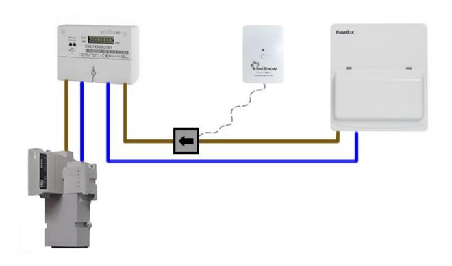
The wireless CT transmitted box should be mounted on the wall near to the electricity meter. The CT or Current Transformer clamp should then be installed with the arrow pointing toward the electricity meter.
