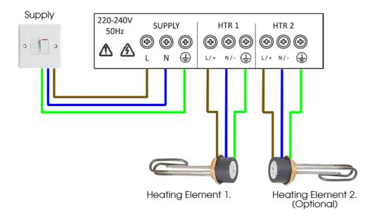
Heating elements to be connected as above.
