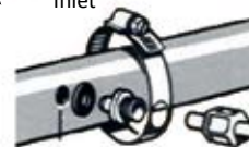
3/8" Hole Saddle Clamp Assembly system piping
