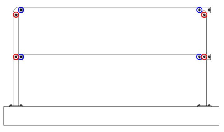
**STEP 7** Tighten the grub screws in the blue circles first. Then tighten the grub screw in the red circles.
