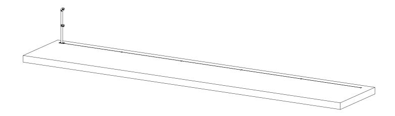
**STEP 4** After mounting the post using concrete fasteners attach the starter fittings.
