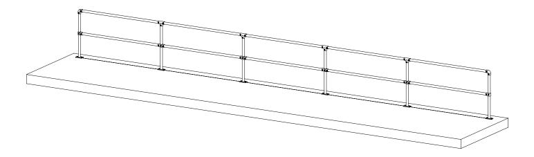
STEP 8 Repeat step 5 to step 7 until handrail is completed.
