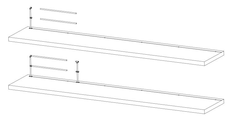
**STEP** 6 Install the horizontal tubes and second vertical post.
