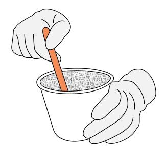
Measure out material into mixing cup by **VOLUME** 1A:2B, or by WEIGHT 64A:100B See the Quick Mix Guide for amounts.
