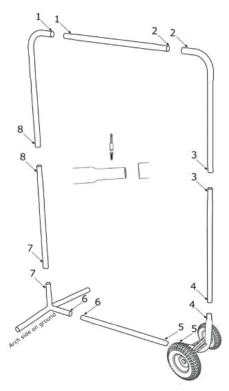
Arch should be positioned to set on the ground to accommodate uneven surfaces. Flip or turn it until you have it positioned correctly.
