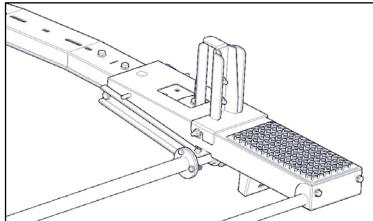
• If using an "Extension Ladder" put the Ladder Stop(I) at the same location on the Front & Rear Bow Assy.(A&B).
