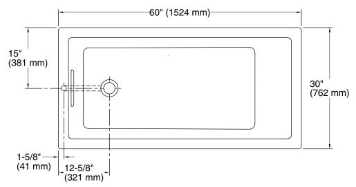
No change in measurement if connected with drain illustrated. (K-7272)
