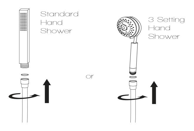
**Step 2A** Finally, install the hand shower to the hose, as shown.
