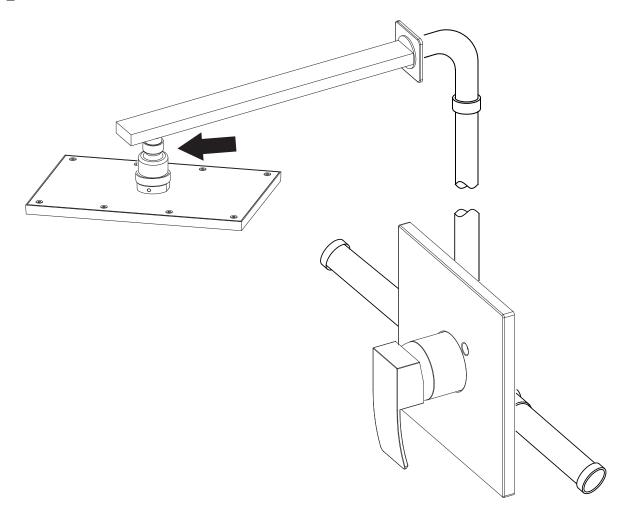
**FINAL** Check the connections pointed by the arrows for any kind of leaks and re-tighten if necessary.
