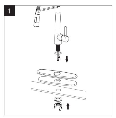
1. Position the faucet in order on the counter top as shown. Don't forget the O-ring. Assemble gasket assembly and lock nut to faucet threaded sleeve by hand and tighten the screws with screwdriver.
