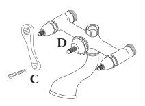
Install the handles. Be sure the broach screws (E) are tightened before installing handles.
