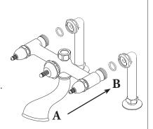
Thread the brass nipple into the supply shank (B).
