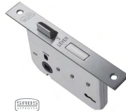
QS5757 Stainless steel forend – three lever 57mm backset 57mm centre
