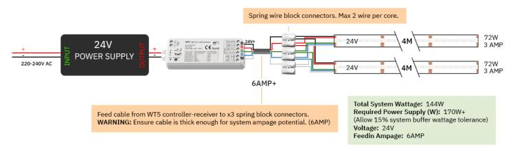
Typical Wiring Setup: Mains > 24V Power Supply > <u>WT5 Controller-Receiver</u> > <u>5 Core Flat Feed cable</u> (<u>Check Amps Needed</u>) > Spring Connectors > <u>RGBW COB LED Tape Lights</u> ((( <u>Wireless 4 Zone Remote</u>
