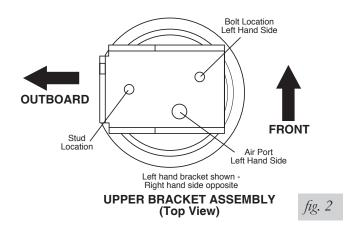
4. Set roll plate on bottom of bellows. Attach lower bracket to bottom of bellows on both units using the holes as shown (Figure 1). The extended tabs should face rearward. Use the 3/8" lockwashers and 3/8-24x7/8" HHCS torque to 15-20 ft.-lbs. Be sure that lower bracket and upper bracket are parallel to each other as shown in Figure 2.
