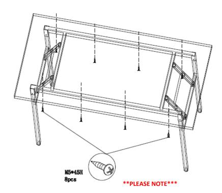
Supplied timber top attaching screws are for use with top thicknesses of 25mm or greater. Do not use these screws if your top thickness is less than 25mm
