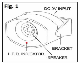
**Step 1** Choose a spot to set your EZ-Mount that is closest to the Rodent Problem. At the same time position/aim the device facing the most open area of that room or area. This good, open coverage allows the sounds to fully cover the area.
