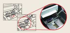
The effect of the automatic cleaning is reduced when wipers are worn. Check wipers on a regular basis to ensure their performance.
