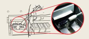
Dirt around the wipers may lower the effect of the automatic cleaning and can also be a factor of damaging the print heads.
