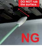
Rough cleaning may damage the print head's water-repellent coating and worsen the problem.
