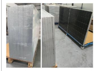
3 Modules are added and the Stretch Wrapping Process is
