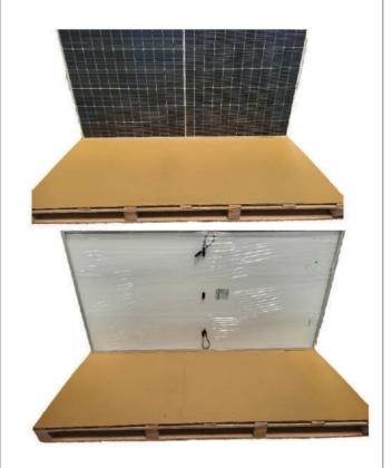
STEP 2: First Panel is placed facing Inside followed by Second Panel Facing the First Panel, on the pallet, followed by Stretch Wrapping the first two Panels.
