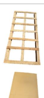
STEP 1: The Pallet is placed on the ground, followed by Placing the Bottom Sheet.
