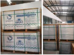
Cut all the Green Pet Straps. Remove all the L Angle Production Boards The Stretch Wrapping of the modules will keep the Pallet assembly intact.
