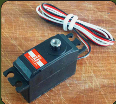
Quality metal gear servos are included in the kit as standard but need their mounting hole plate removed to fit in the servo bays.
