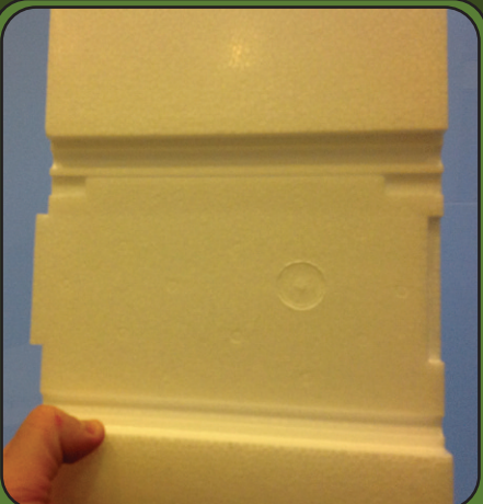
You can clearly see the servo channel moulded in to the wing extension here. I removed this for ease of swapping out the long wing to the short wing as it meant one less servo extension.
