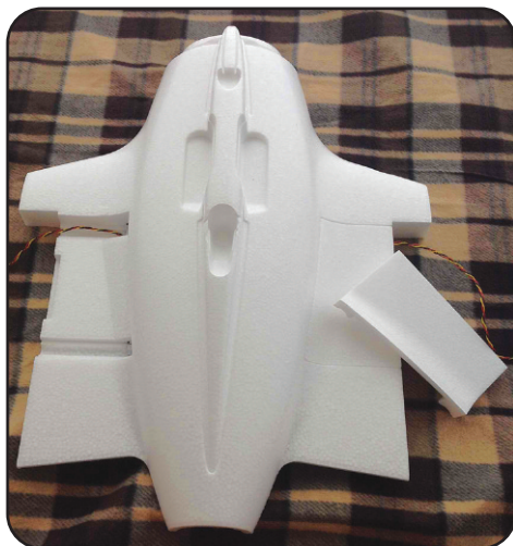
Here you can see the right side of the fuselage completed and sealed with the left ready to seal.
