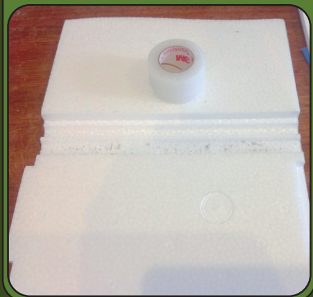
You can clearly see the servo channel moulded in to the wing extension here. I removed this for ease of swapping out the long wing to the short wing as it meant one less servo extension.
