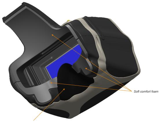
Black anti reflection area (part of the bottom plastic cover) This nose area stops the internal lens and display from fogging by direction down the exhalation air. It is painted black to avoid light reflections
