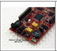
If you use GoPro connector with OSD then set jumper Camera Voltage regulator to
