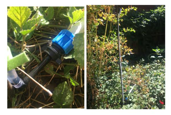
Attach IG16217 Measuring tool to the end of a BluSoak tape line. If with a good valve (globe valves hardest to find but work the best) you can adjust the water level in the tube until it's 2-3' up. At that point, the soaker hose when on will use about  $\frac{1}{4}$  gallon per foot per 24 hours. The amount of water is in the same ratio as the water level – e.g. if you double the height, you will double the water flow.
