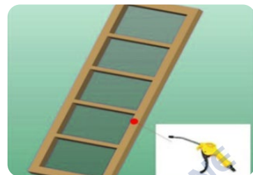
Clean the shaker screen with an air blower
