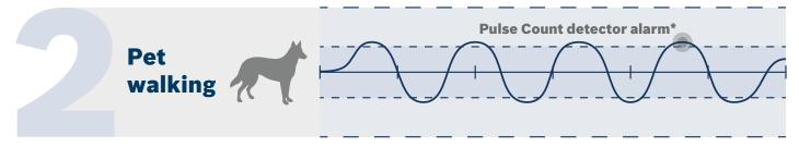
**Bosch detector ignores source; Competitor sends false alarm** \*Pulse count set to 4
