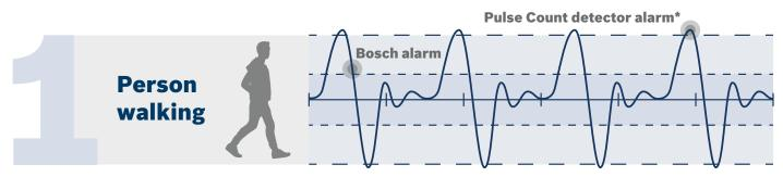
**Bosch detector alarms at first zone; Competitor alarm is delayed** \*Pulse count set to 4
