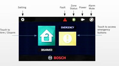
The ICP-CP4TS 4.3" Touchscreen is an entry level codepad for the Solution Ultima 844/880 intrusion panel. Designed to mimic the functionality of the ICP-CP508W Icon keypad while also providing the flexibility and ergonomics of a modern touchscreen, the ICP-CP4TS allows for both convenient use and full programming of the intrusion panel. The simplistic user interface is both easy to navigate for the end user, and familiar to operate for the installer.
