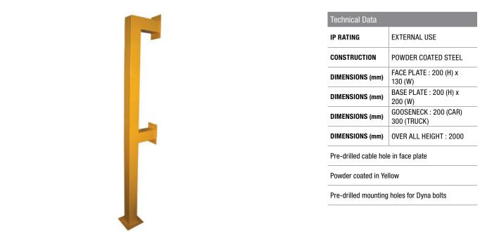
2000mm Straight bollard with truck and car goose neck and intercom or access control face plates. Sand blasted and powder coated in yellow.
